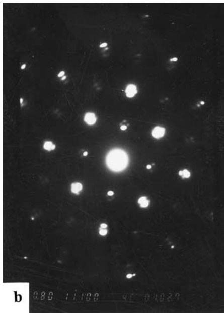
Figure 6 TEM bright-field image (a) and SAED pattern (b) of melt-spun Al-10 Sr alloy quenched at the wheel speed of 1800 rpm.
